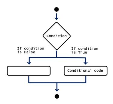
The graph could help you imagine the process of the conditionals. Before it displays the outcome of the operation, the machine follows these logical steps. If the conditional code is not to be executed because the if-condition is not true, the program will directly lead you to some other output or, as it is in this case, to nothing. After any of the two situations, the machine will go to the next black point and will progress from there on.
