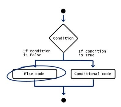
Instead of leading to no output, if the condition is false, we will get to an else code. Regardless whether the initial condition is satisfied, we will get to the end point, so the computer has concluded the entire operation and is ready to execute a new one.
